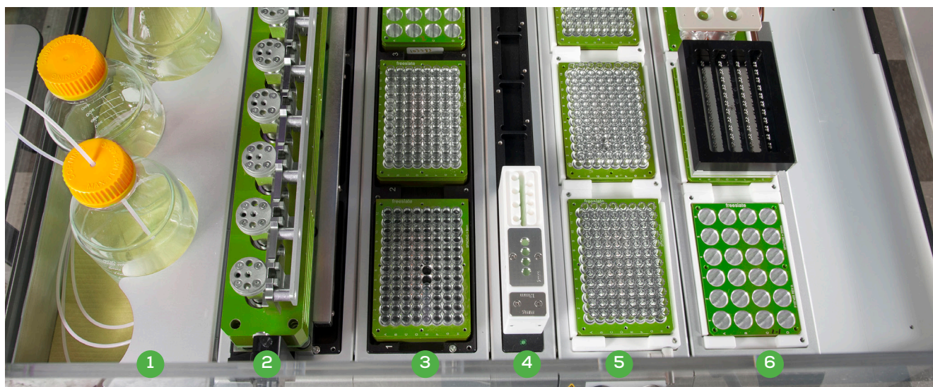
Figure 6: The Junior deck layout. (1) solvent tray, (2) OSR, (3) 3-position passive rack, (4) wash station, (5) heating/cooling/stirring station and (6) heating/stirring station.
