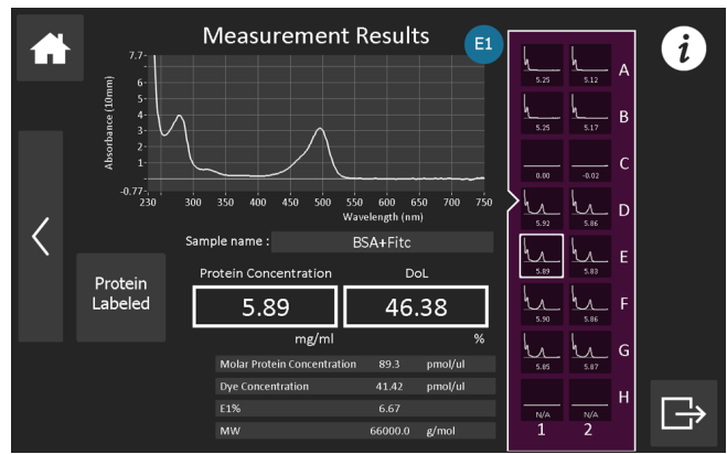
Figure 4: Illustration of the Results screen on the Little Lunatic.
