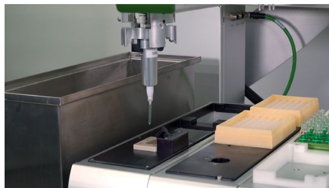
Figure 1: A Big Kahuna or a Junior (pictured) with a viscosity station automates low volume, high-throughput viscosity measurements.
